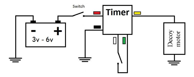
Connect the decoy timer according to the diagram.
