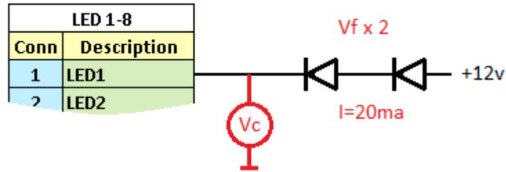
With  $V_f = 3\text{v}$  the  $V_c = 12\text{v} - 3\text{v} \times 2 = 6\text{v}$ . The voltage is too far from target  $0.6\text{v}$  so it needs to be lowered. To lower the  $V_c$  voltage resistor has to be added.
