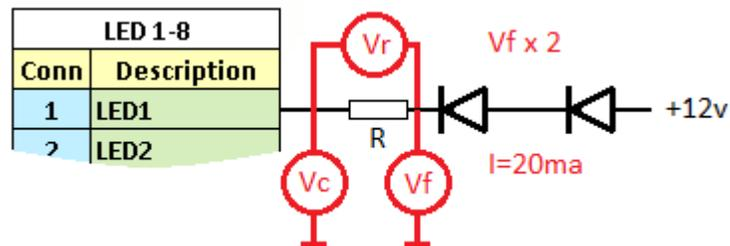
$V_f$  is equal  $12\text{v} - 3\text{v} \times 2 = 6\text{v}$ . The  $V_c$  target is  $0.6\text{v}$  so the voltage drop on the resistor we need to achieve  $V_r = 6\text{v} - 0.6\text{v} = 5.4\text{v}$ . Knowing the current going through the resistor is the same as through the LEDs  $I = 20\text{ma}$  and the voltage drop we need to achieve we can employ Ohms Law ( $I = U/R$ ) to find the resistance  $R$ .  $R = U/I = 5.4\text{v}/0.020\text{a} = 270$  Ohms.
