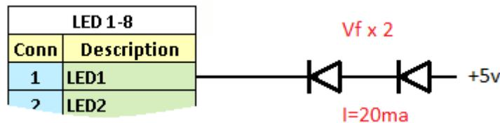
If the  $V_f$  for a selected LED is 2.2v then total Voltage Drop is 4.4v. That makes  $V_c = 5v - 4.4v = 0.6v$  which within our target. If the selected LEDs have  $V_f=3v$  then Voltage Drop will be  $3v*2=6v$  which is higher than supplied 5v voltage and LED will never be fully lit. In that case LEDs should be connected to a higher voltage source.
