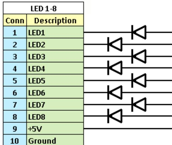
Connecting more than one LED per channel is also pretty simple but takes a little consideration. LED has what it called Forward Voltage or Voltage Drop. Forward voltage defines how many volts need to be applied to the LED for it to light up. The voltage values are between 1.2v and 4v and depend on LED color and manufacturing process. The forward voltage can be found on LED data sheet.
