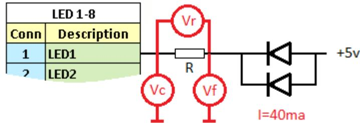
Let's calculate resistor needed for this scenario.  $V_f = 5v - 3v = 2v$ .  $V_c$  target is  $0.6v$  so  $V_r = 2v - 0.6v = 1.4v$ .  $R = U/I = 1.4/0.04 = 35 \text{ Ohms}$ .
