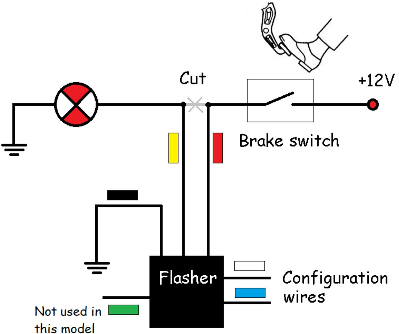
3. Now using provided quick splice connector attach flasher module **BLACK** wire to the **ground** wire.
