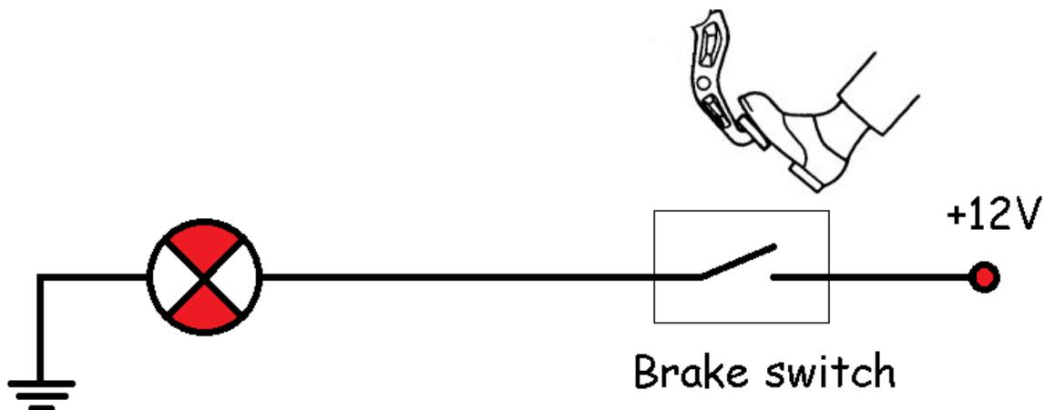
2. Cut the **power** wire and connect flasher module **RED** wire to it. Make sure you use **power** wire end going to the switch and not the bulb.
